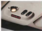
A special courtesy side light gives the front door passenger a glimpse without disturbing the driver.
