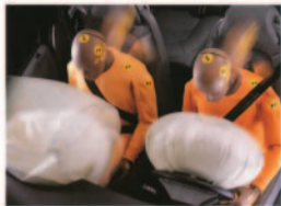
Dual air bags supplement the front safety belts, adding to a few hundredths of a second or so before the driver is propelled forward and upper-body support is lost. The steering wheel is shifted back. Safety is enhanced by generous interior space and adjustable upper-pull-down and automatic retractors for the front safety belts.
