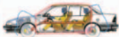
When you ride in a Saab 9000, you are protected by large front and rear crumple zones. The body panels are designed to absorb the initial impact according to a predetermined pattern.
